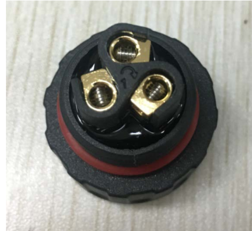
Fig.12. Definition of the AC connector
